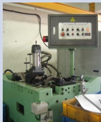
SHF-40 Max. diameter x Thickness : \Phi 40 \times 2.0 Length : 20~6,000mm
