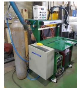
Automatic welding unit
