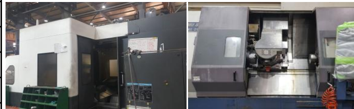
CNC LATHE WITH MILLING HEAD AND COUNTERSPINDLE
