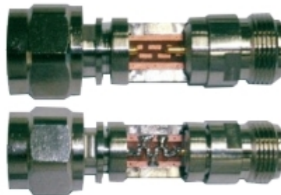
LPF by using Lumped-elements
